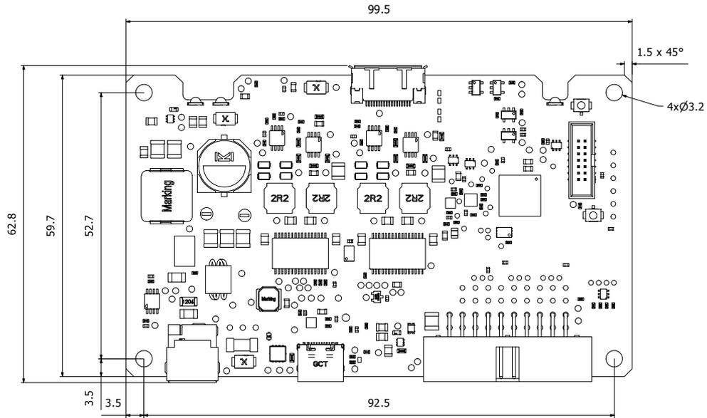
Figure 1: Mechanical drawing of the MR-E-3 base unit board (unit: mm).
