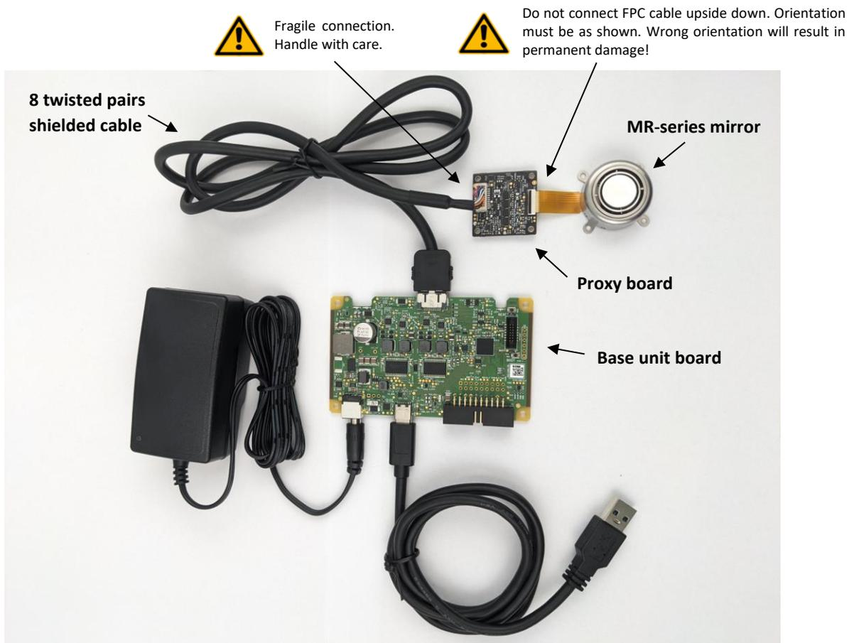
Figure 4: Schematics of correct mirror and board connection.
