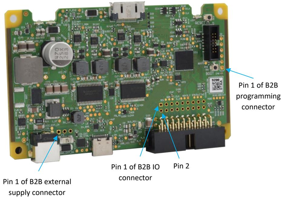
Figure 6: Pin assignments of the B2B connectors.
